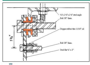
Joel H. Goodman, Consulting P.O. Box 14 Dodgeville, WI 53533 E-mail: joelhgoodman9@hotmail.com Detail section at press fit bearing in vertical plate with rotating steel angle PV beam support seat clamp and over rotation stopper for 1-axis tracking PV pergola.
